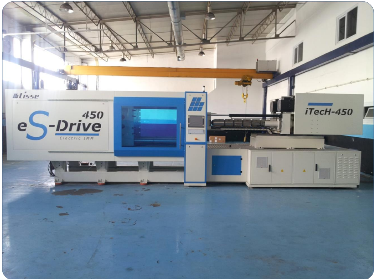
eS-Drive450 Tisse machine, the first Hybrid Machine in plastic injection molding: speed and energy saving
